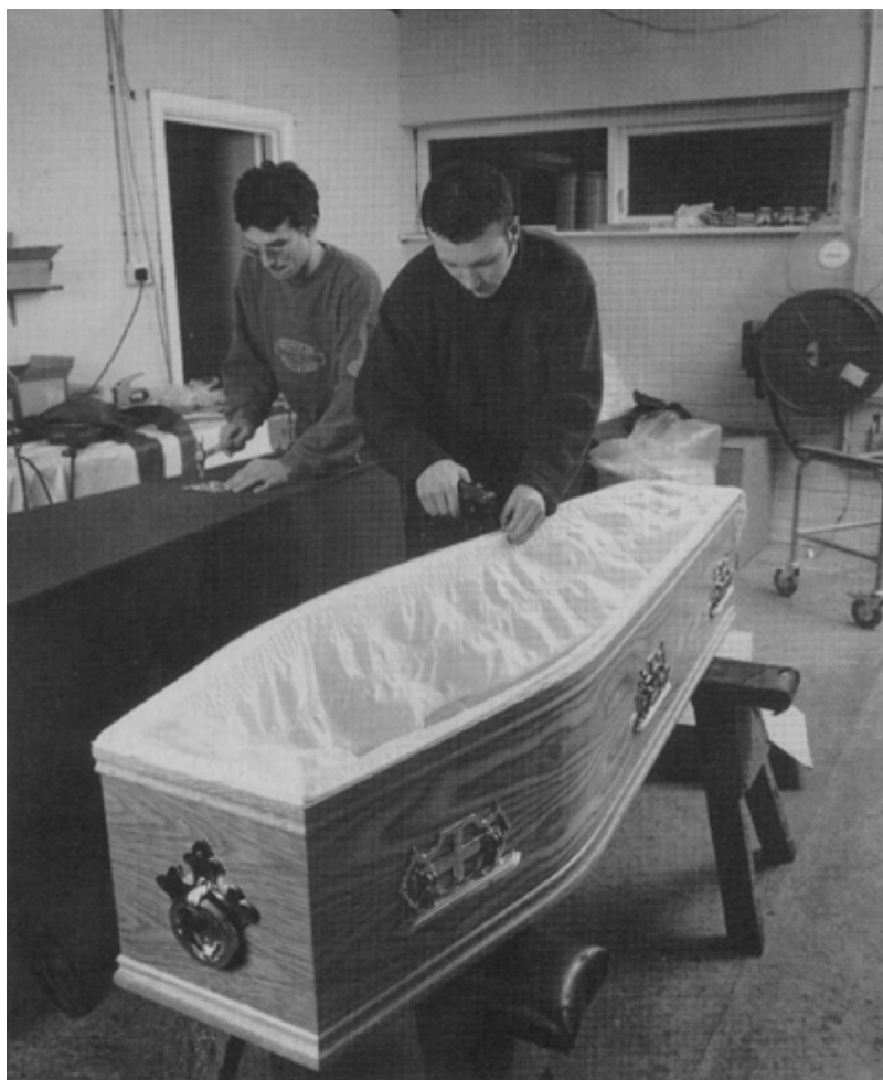
3. The coffin workshop Linings and fittings are being stapled and hammered in place. First lined with bitumen and polythene, the coffins are then embellished with satin and lace. Work proceeded to the beat of the radio. The notice board in this parlour was covered with letters of thanks from relatives.
